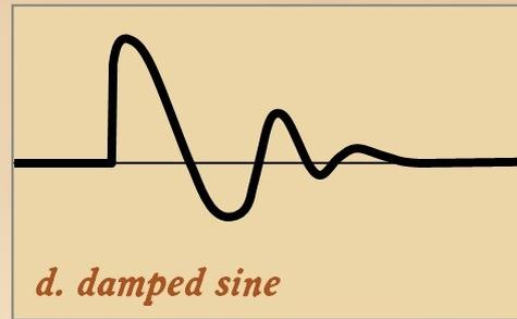
Compensatory reactions overshoot target, oscillating during the decay back to reference.
