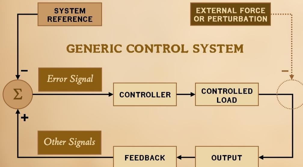
**CLOSED LOOP CONTROL SYSTEMS** react to correct differences between actual state and a reference value.
