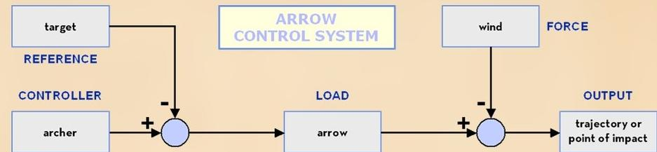
**ARROW:** No feedback - open loop. Course cannot be assessed nor corrected. Must be calibrated (aimed), and if a gust of wind or anything upsets that calibration, the system misses its mark.
