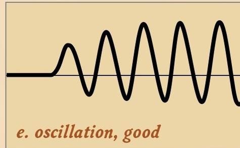
Overshoot goes back-and-forth, creating oscillations. This can be intentional or desirable, as in clocks or radio wave circuits.
