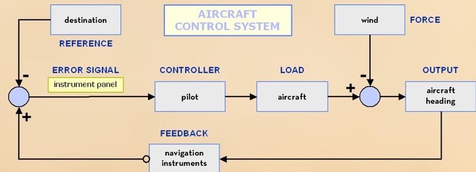
**AIRPLANE:** Steered, not aimed. Pilot and flight controls assess and correct the plane's heading. Feedback and closed loop control assure that system reaches target, even when perturbed.
